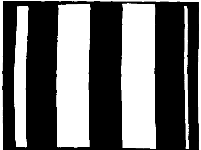
FIGURE 7.4-1 SIGNAL 64H The simplest way to achieve a video display is to couple a sync output to the video line.
